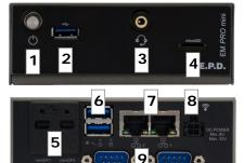
**On/Off**(1) - press the power button 1x to turn the computer on or off. Press and hold it for more than 4 seconds to force a power off.
